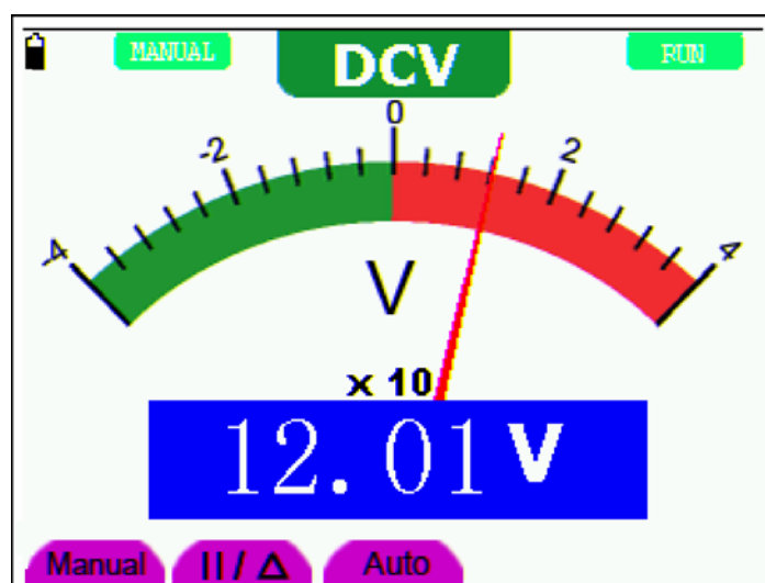
Figure 33: Automatic/Manual Range Adjustment
