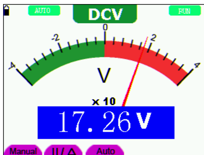
Figure 25: DC Voltage Measurement
