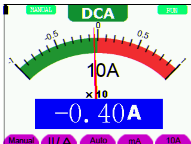
figure 28: DC Current Measurement for 10A
