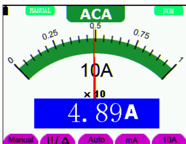
figure 30: AC Current Measurement for 10A
