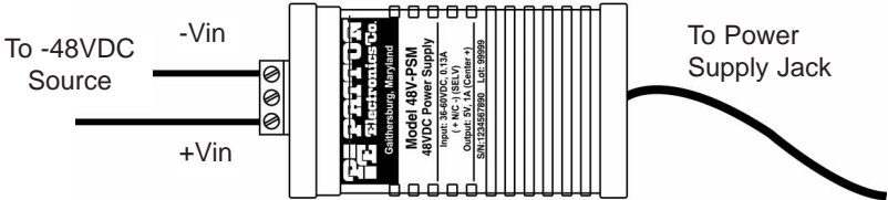
Figure 9. Connect DC power to the 48V-PSM DC power supply
