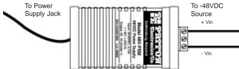
Figure 5: Connecting DC Power to the 2701 DC Power Supply.
