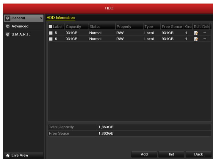
Figure 10.4 HDD Status Changes to Normal
