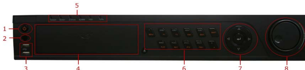
Figure 1.1 DS-7300HI-ST&DS-7300HFI-ST Front Panel
