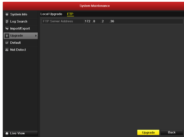
Figure 12.13 FTP Upgrade Interface
