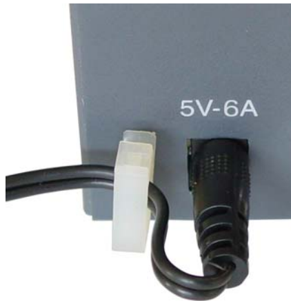
Figure 8. Connection of the DC Input Jack
