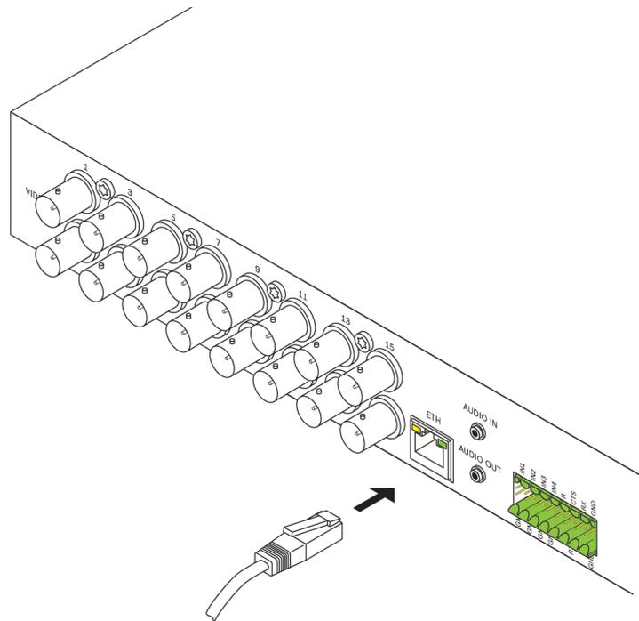
You can connect the VIP X16 XF E encoder to a 10/100/1000 Base-T network using a standard UTP category 5 cable with RJ45 plugs.
