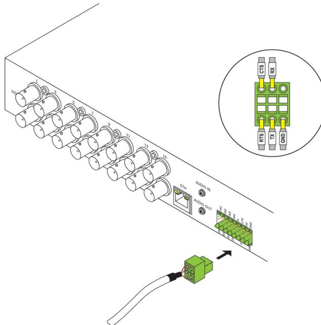
The bidirectional data interface is used to control units connected to the VIP X16 XF E encoder, such as a dome camera with a motorized lens. The connection supports the RS-232, RS-422, and RS-485 transmission standards. A video connection is necessary to transmit transparent data.
