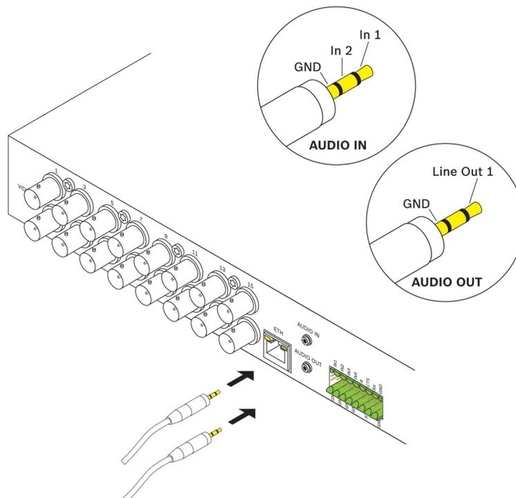
The VIP X16 XF E encoder has two audio ports for audio line signals.
