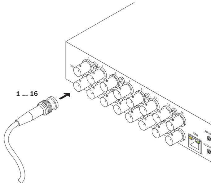
You can connect a maximum of 16 video sources to the VIP X16 XF E encoder. Any cameras and other video sources that produce a standard PAL or NTSC signal are suitable.
