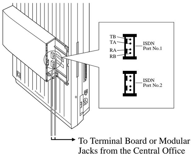
11. Fix the cords to the wall as shown so that the front cover can be opened.
