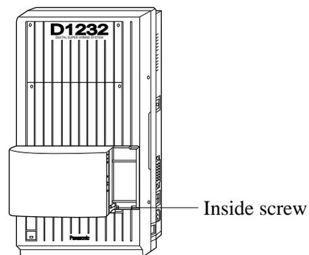
**Note** Be sure to fix the inside screw to the main unit, or the unit may not work properly.
