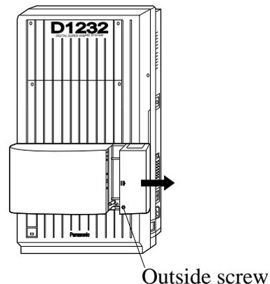
5. Secure the inside screw (included) to fix the cabinet to the main unit.
