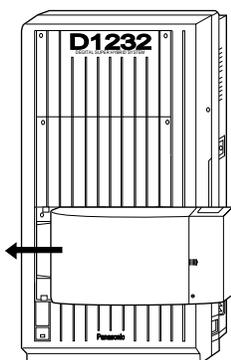
4. Loosen the outside screw and slide the cover to the right.
