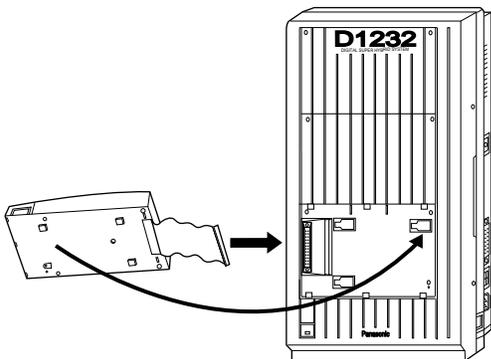
3. Hook the cabinet to the main unit and slide the cabinet to the left until it is secured.
