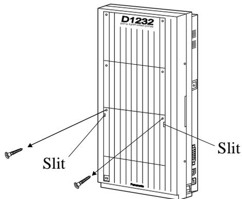
**Note** Any of the cover plates can be removed, as needed.
