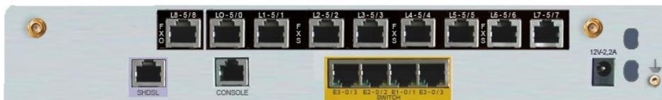
Figure 4. Rear panel with 8 FXS and 1 FXO
