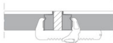
Fig. 18.6 Detailed view of the Uni-assembly lock
