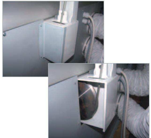
Figure 38.3: Upper rope holder with and without cover
