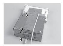
Remove the two screws (Torx T-20) in the bottom of the electronic unit and store them in a safe place. Align the terminal holder exactly with the two holes and secure it with the Torx T-20 countersunk head screws (G).
