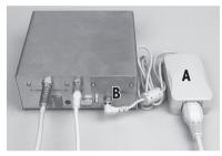
Connect the AC adapter (A) to the connector (B) on the back of the electronic unit and to your power supply. Tighten the connector to ensure a good connection to the electronic unit.
