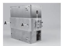
Remove the two existing screws from the bottom side of the electronic unit (Torx T-20) and use the provided Torx T-20 countersunk head screws (A) to secure the mounting bracket.
