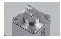
Put the **standard weighing pan** (D) onto the weighing pan adapter.
