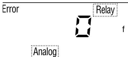
To acknowledge the error message at least 4 mA must be applied at the signal current input, then the pump starts up again independently and the error message "Error" and the flashing "Analog" go out.
