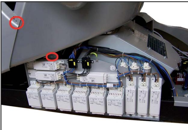
With some units, the lower part of the seat cover is also screwed under the upper part of the seat cover. If this is the case, also remove these screws. Then remove the cover from the tanner.
