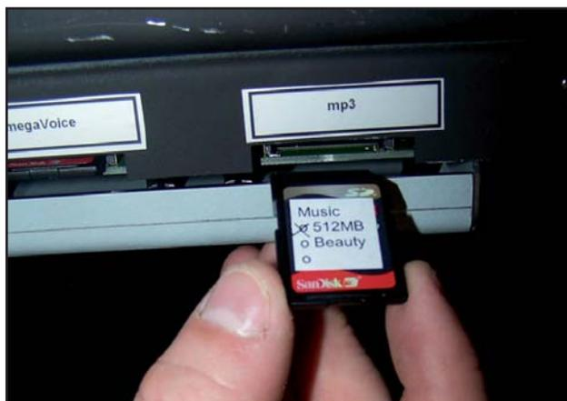
5. Re-start the device. To do so, pull out the main plug and plug it in again. In this way, you make sure that the MP3 player will identify the SD card.
