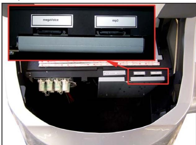
4. Insert the SD card, fasten the covering plate and the seating surface.
