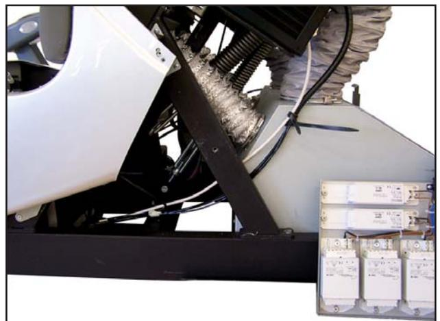
7. Tighten the two springs of the upper-body tanner in such a way that the canopy part remains still and stable in any position (1 = springs, 2 = tensioner).
