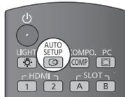
When **AUTO SETUP** on the remote control is pressed, "Auto Setup" will be executed.
