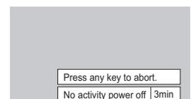
When the power is turned off due to this function, a message "Last turn off due to 'No activity power off'." is displayed next time the power is turned on.
