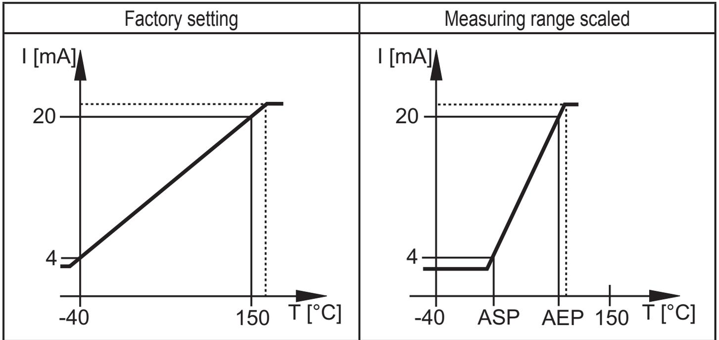
In the set measuring range the output signal is between 4 and 20 mA.
