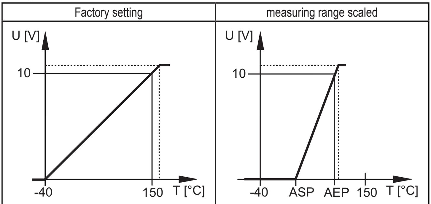
In the set measuring range the output signal is between 0 and 10V.
