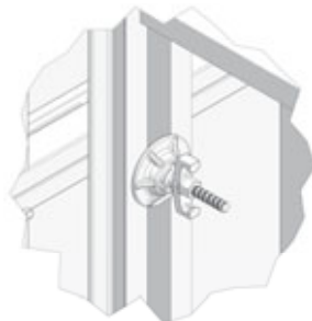
Fig. 4.4 Detail - Fixing screw at the side of the STB
