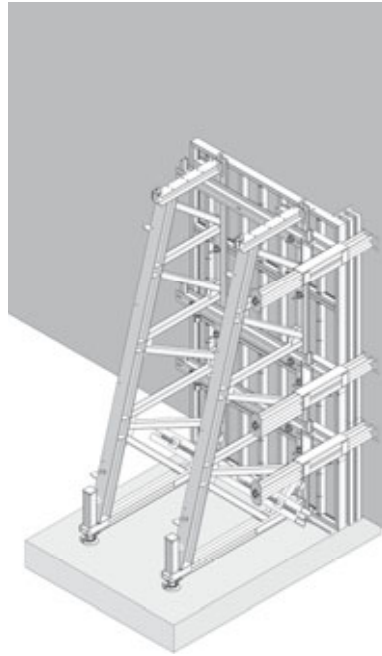
Fig. 15.2 An STB 450 requires 3 stop end brackets
