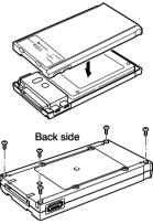
Use a No. 0 Phillips screwdriver to secure the screws.
