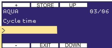
Defines the aquaCool and aroma cycle time (spraying time + spraying interval).
