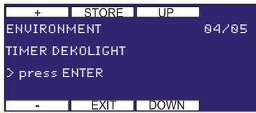
Entering switching times for the decorative lighting. The submenu is invoked by pressing START (ENTER).
