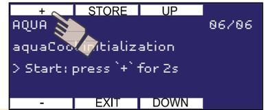
Starts the aquaCool initialization process. A spraying cycle of 90 seconds is started to bleed the system before commissioning, after a repair operation or after a canister replacement.
