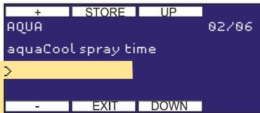
Determines the duration of the aquaCool spraying time.
