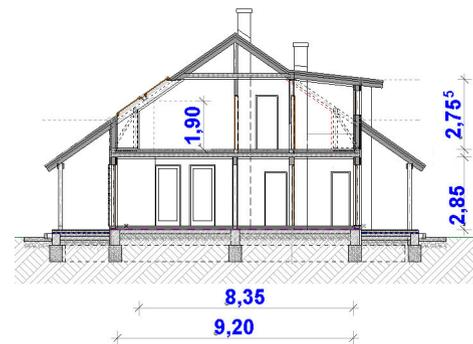
ArchiCAD's numerous helpful conventional documentation tools, such as dimension markers, zone stamps or fills with area markers turned on, help the user to obtain the necessary height and area data quickly, from which the building volume may easily be calculated.
