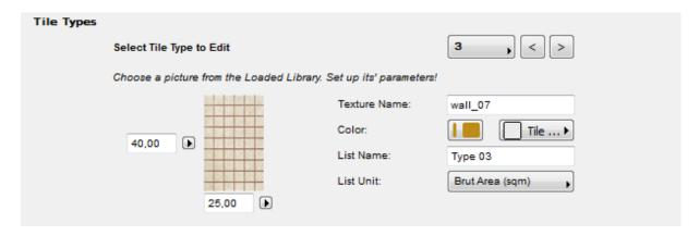
**Select Tile Type to Edit**: each tile type has got a number. You will edit the setting of the tile type with the chosen number. The number of tile types range from 1-8 in the full version of the solution. The default tile is always number 1; this will be used to make the base tiling of the building element. The assembled palette can be used to change the color or texture of tile rows and individual tiles. (see: *4.2.2 Tile View Mode*).
