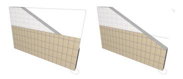
**Use Bottom Contour**: mark this checkbox to trace the bottom edge of the wall if the edge is not straight. If this option is switched off the Add-On will complete the tiled surfaces to a rectangle.
