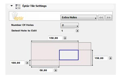
There is no need to tile surfaces behind plumbing fixtures, for example bathtubs. Use extra holes to create untiled patches on your wall. These holes only appear in the tiled surface, they do not affect the wall. To create holes in both the tiles and the wall use ArchiCAD openings. Extra holes on the walls can only be rectangular.
