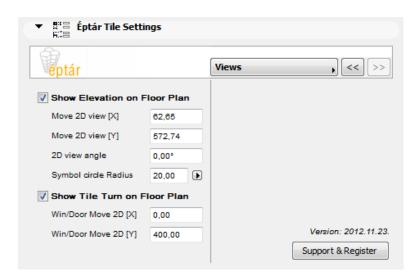
This tab page can only be found for walls. The checkboxes and fields enable us to choose which views we want to display on the floor plan and where we want to position these views. Position can be set here on this page but we can also change it on the floor plan, with moving hotspots (see: 4.2.1 Geometry)
