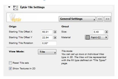
**Origin**: the default place of the origin of the tiled surface is in the corner marked with the circle. The place of the origin can be edited either in this window or on the 2D and 3D views (see:
