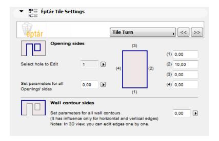
Tile Turn options are used to define the tiling of door and window sills and wall edges. Tile Turns can only be set in Add-On mode.
