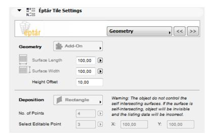
**Geometry**: in Add-On mode you can only modify Height offset. For slanted floor surfaces use individual placement (7 Individual Placement).
