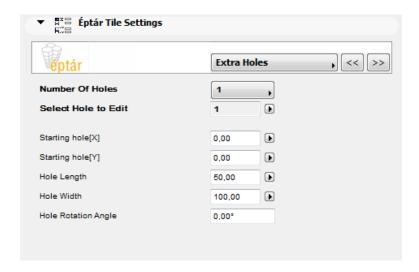
You can leave out the area under plumbing fixtures from the tiling by defining extra holes on the tiled surface.
