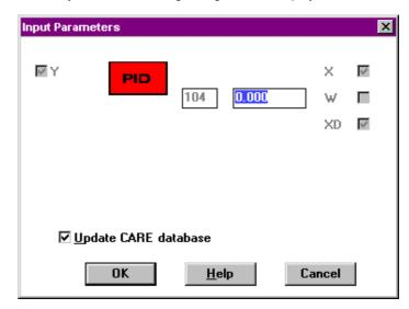
NOTE: The dialog box is the same as in Excel CARE except for the addition of the Update CARE database check box. If this box has a checkmark, Live CARE writes any changes you make to the CARE database when you click **OK**. If the box does not have a checkmark, changes you make are not saved in the database, when you leave Live CARE.
