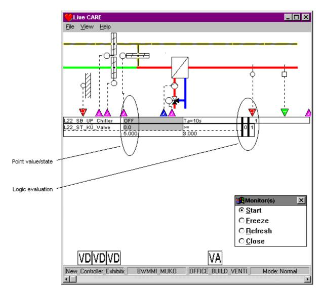
**5.** To fix a switching table point, click point value/state in the gray area in the switching table. See the Fix/Unfix Points section for more information.
