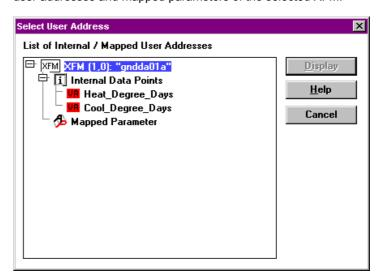
If there are no internal data points and/or mapped parameters available for the desired XFM the Internal Data Points and/or Mapped Parameters structure is not expanded.
