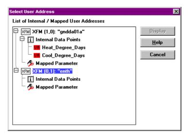
For Internal user addresses and mapped parameters their type, such as VA or VD, and their name, such as Heat\_Degree-Days or P08\_Factor are shown.
