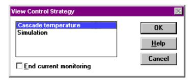
If no control loop was previously selected for the current plant, the first loop in the list is automatically selected. Otherwise, the last control loop viewed is highlighted.
