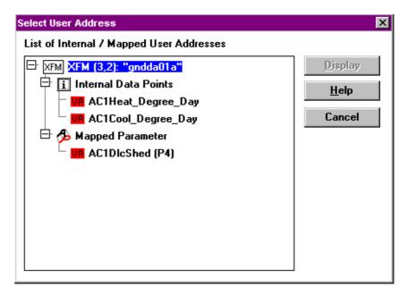
The XFM is displayed prefixed by the position of the XFM in the control strategy (column, row). If there are no internal data points and/or mapped parameters available for the desired XFM the Internal Data Points and/or Mapped Parameters structure is not expanded.
