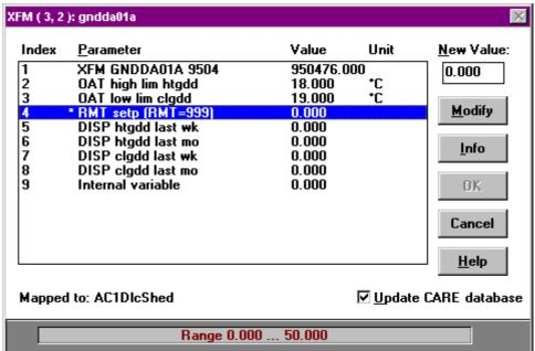
Note that the dialog boxes are the same as in Excel CARE except for the addition of the Update CARE database check box. If this box has a checkmark, Live CARE writes any changes you make to the CARE database when you click **OK**. If the box does not have a checkmark, changes you make are not saved in the database, when you leave Live CARE.
