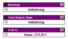
3. Click Start in the simulation software window at the bottom of the screen when Static Simulator was selected for the communication interface. When directly communicating with a controller via the B-Port or LonWorks communication interface monitoring starts automatically after initializing.
