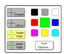
Points are captured by aligning the tool over the edge of the feature being measured and pressing enter to register the point. Points can be automatically captured, by leaving the tool stationary over the feature for a preset time (seconds).
