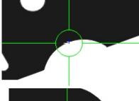
The multiedge tool is used to capture multiple points either inside or outside the field of view. For inside the field of view position the tool in the centre of the feature being measured, press enter to fire the points.
