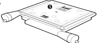
► Check the top of the adapter **6** and the underside of the stage are clean and free of any debris.
