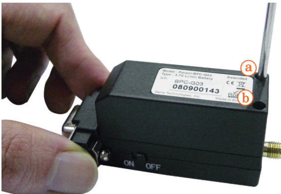
Figure 2-7 Fasten the battery pack
