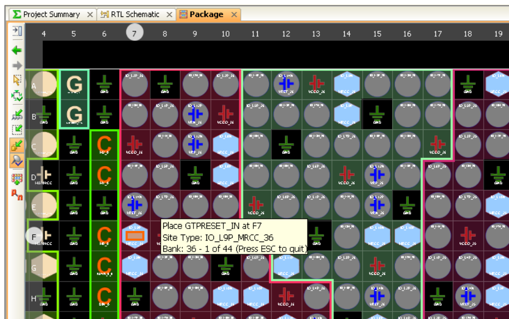
Figure 8-20: Placing I/O Ports Sequentially
