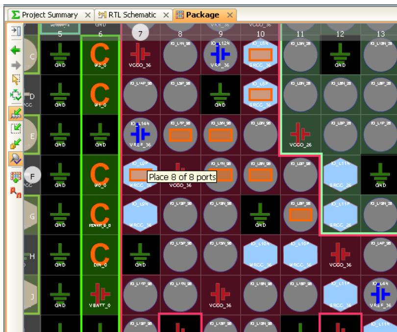
Figure 8-21: Placing I/O Ports in I/O Banks
