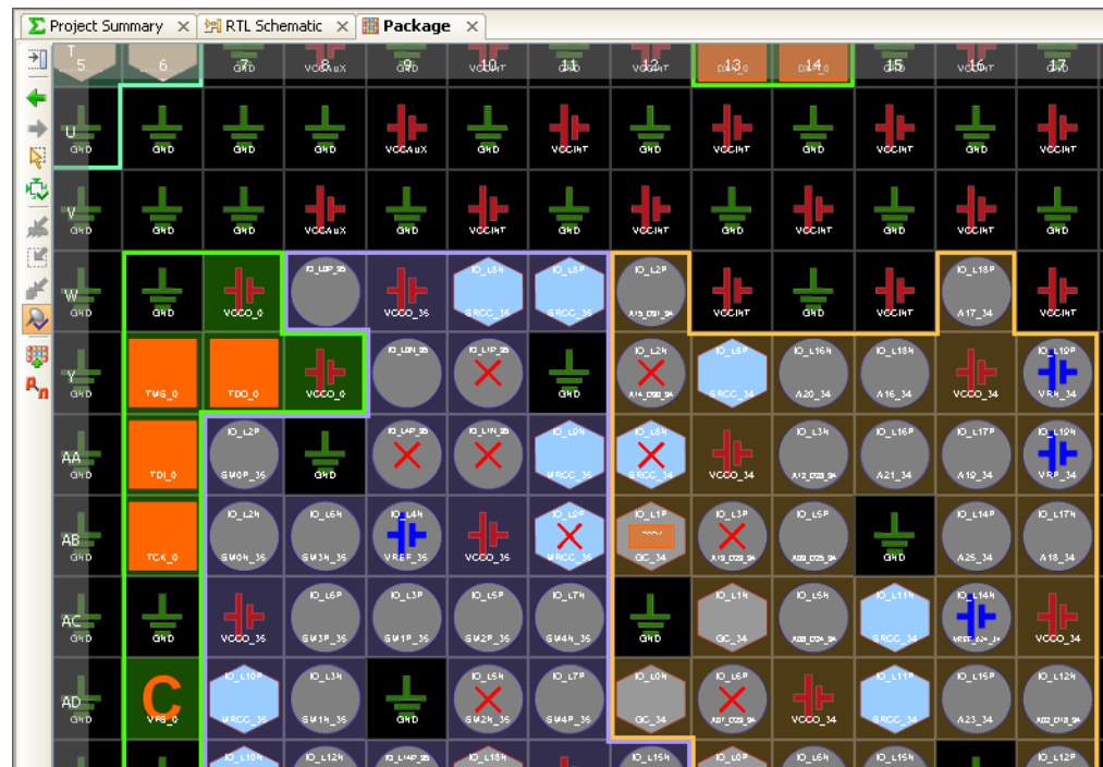
Figure 8-17: Setting Prohibits on Package Pins
