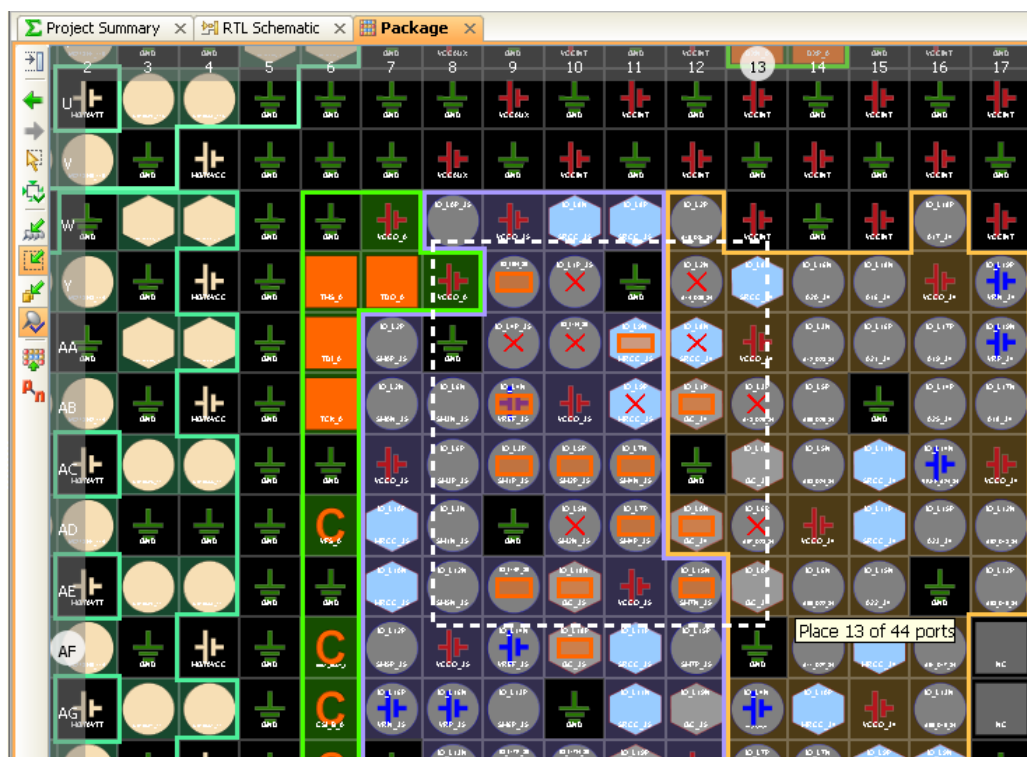
Figure 8-22: Placing I/O Ports in an Area
