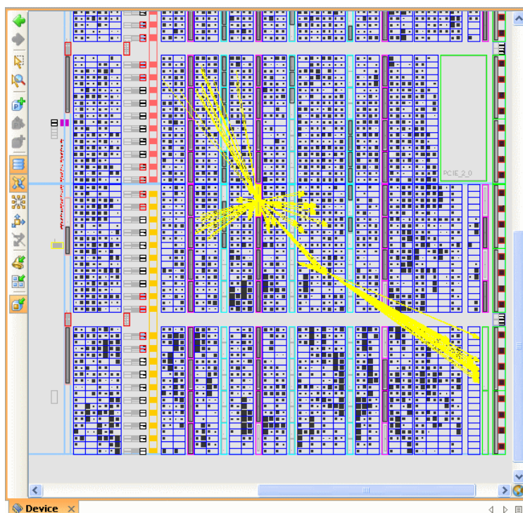
Figure 11-12: Net Connectivity in the Device View
