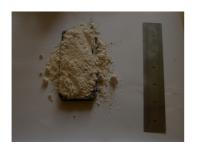
**Step 3.** Press the flour into the box with the flat surface of the ruler in order to compact it. (Please hold the ruler lengthwise.)
