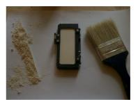
**Step 7.** Hold the closed box in your left hand (possibly without touching the glasses) and clean it with the brush. Take the sample holder in your right hand and put the box under the springs in that way, that the box goes into its place.
