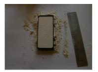
**Step 6**. Lift the box carefully and remove the needless quantity of flour from the paper sheet. Afterwards, place the box back on the paper sheet and clean it at the hinges. Then put its cover aside and join them up at the hinges (with moving the parts on the paper sheet). Finally, close the box and the cover with a strong pressure.
