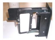
**Step 8.** Put the sample holder into the instrument and push the button for measure.
