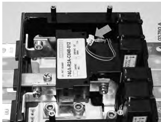
Figure 3: Bypass relay control wires (75 kW ~ 110 kW models)
