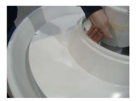
7) Locate the winged pipe clip on the underside of the header tank. Undo the pipe clip and disconnect the tubing from the header tank.
