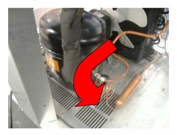
The refrigerant suction pressure remains virtually constant (0.9 bars – 12 psi) during the entire ice making process; it may vary a bit ( $\pm 0.2$  bars – 3 psi) in relation to the water supply temperature variation.
