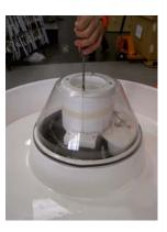
6) Carefully lift out Ice shelf moulding from the centre to reveal the inner of the ice trough moulding.
