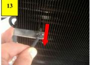
Remove the two m8 fixing bolts fixing the condenser to the base plate. A 10mm spanner will be required for this (pic 14)
