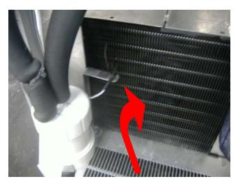
The exhaust hot air, coming from the condenser, is forced to go through the louvers at the back of the machine via the metal shroud that covers the whole assembly.
