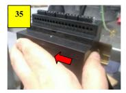
Slide on new Control box and connect all terminals. Important Note: Ensure all cables are connected back in the correct orientation. (Pic 36)
