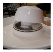
5) Remove the inspection cover by unscrewing the four fixing screws, Lift off inspection cover.
