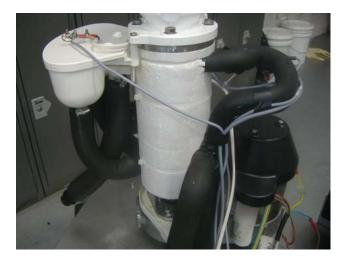
The water constantly flowing into the cylinder bottom part freezes into ice when in contact with the cylinder inner walls. The ice is then lifted up by the rotating auger and compacted and forced out through the opening of the icebreaker and out of the plastic discharge chute.
