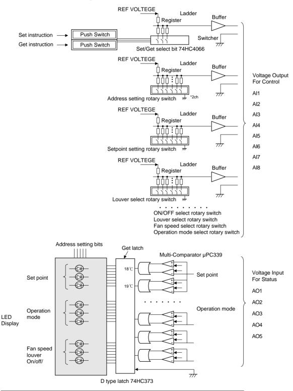
This circuit can be realized by hardware. Design this circuit to maintain the accuracy of voltage output and input detection.
