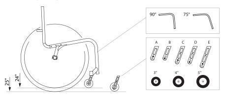
To ensure that the frame is straight and the axles of the front wheel forks are perpendicular to the ground, choose one of the combinations listed in the table.
