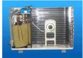
7. Remove middle separate plate and electic. Remove compressorís cover and protector. Remove four-way valve wire.
