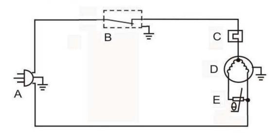
A.POWER PLUG B.THERMOSTAT C.OVERLOAD PROTECTOR D.COMPRESSOR E.PTC
