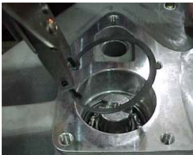
Figure 45. Removing Internal Retaining Ring
