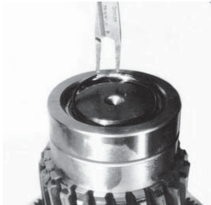
Figure 49. Removing Round Retaining Ring from Input End of Shaft
