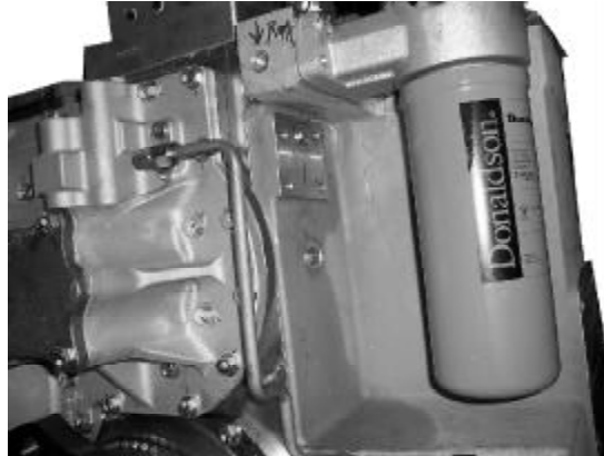
Figure 125. Oil Filter Installed
