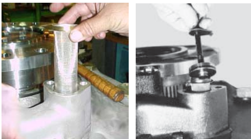
Figure 122. Install Suction Strainer
