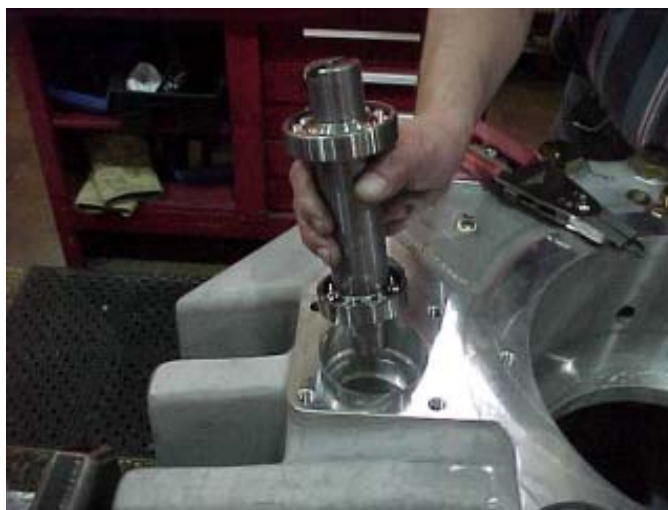
Figure 80. Installing Trailing Pump Shaft
