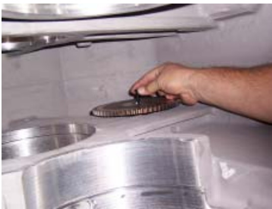
Figure 82. Securing Trailing Pump Gear to Shaft
