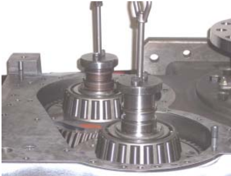
Figure 103. Installing Clutch Shaft Assembly
