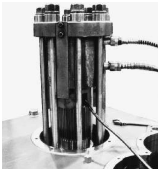
Figure 86. Output Gear Advancing Tools Installed
