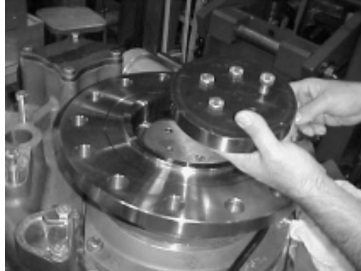
Figure 33. Removing Output Flange Retainer
