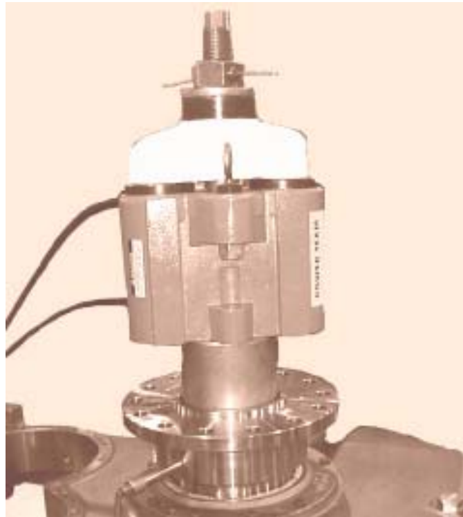
Figure 116. Advancing Output Flange Onto Output Shaft
