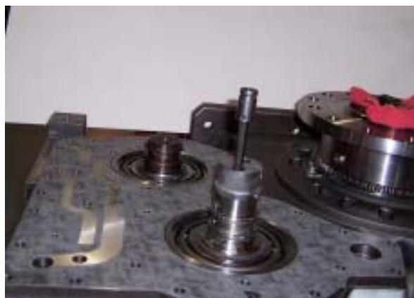
Figure 36. Remove Adapter, Spacers and Shims
