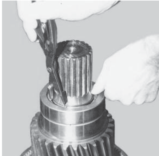
Figure 101. Installing External Retaining Ring Onto Clutch Shaft
