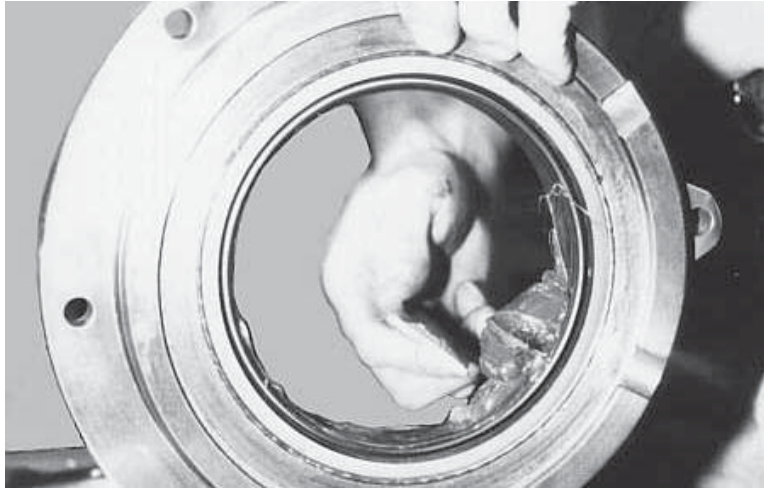
Figure 92. Packing Cavity Between Output Seals With Grease
