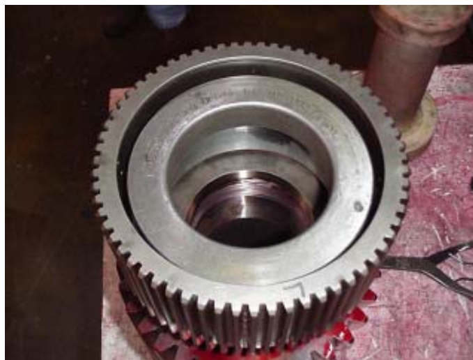
Figure 98. Installing Tapered Roller Bearing Cup Into Pinion
