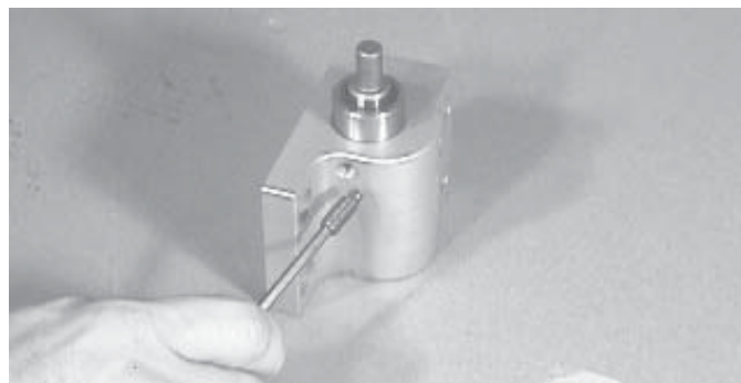
Figure 72. Removing Dogpoint Setscrew
