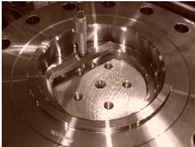
Figure 115. Measuring Output Step Height
