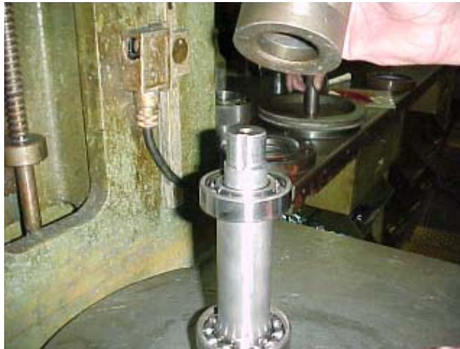
Figure 79. Installing Trailing Pump Shaft Bearings
