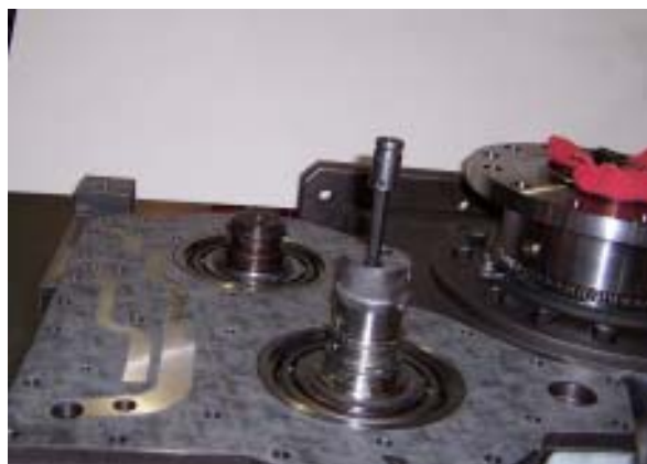
Figure 110. Attach Pump Adapter
