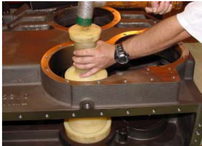
Figure 77. Front Pinion Bearing Cup Installation
