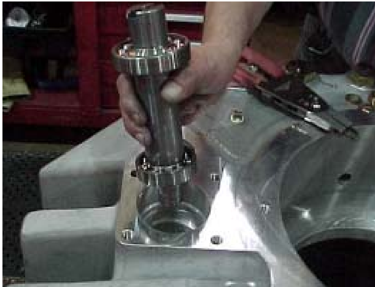
Figure 46. Removing Shaft Assembly
