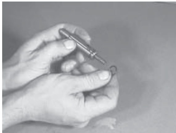
Figure 74. Removing O-ring from Stem
