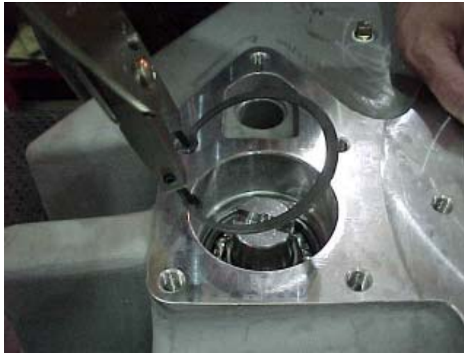
Figure 81. Installing Internal Retaining Ring
