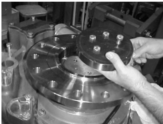
Figure 117. Installing Output Flange Retainer Washer and Shims
