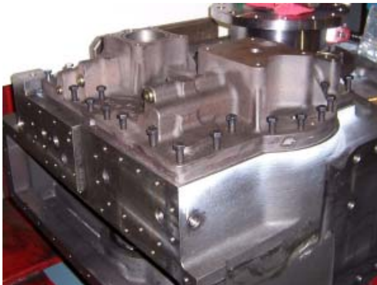
Figure 112. Manifold Attaching Screws
