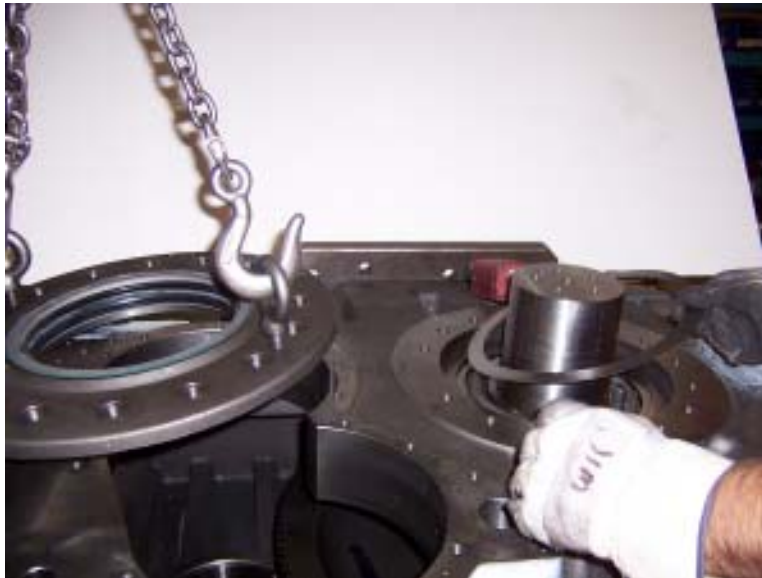
Figure 88. Output Bearing Shims Location
