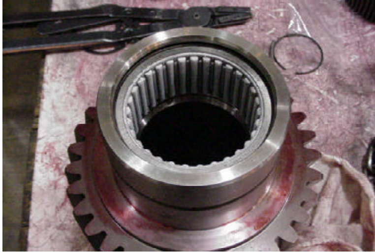
Figure 99. Needle Roller Bearing Installed
