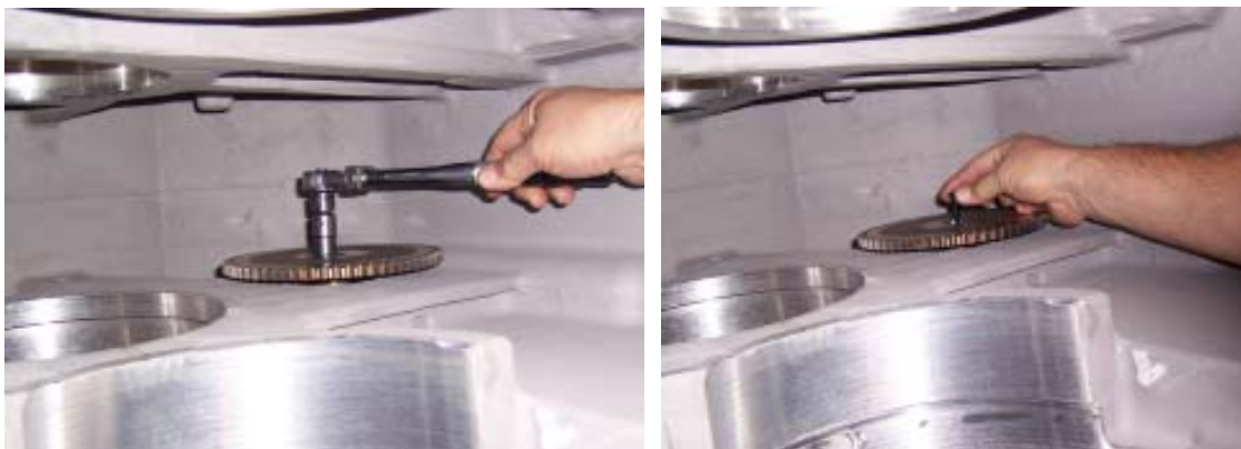
Figure 44. Removing Retaining Cap Screw and Washer
