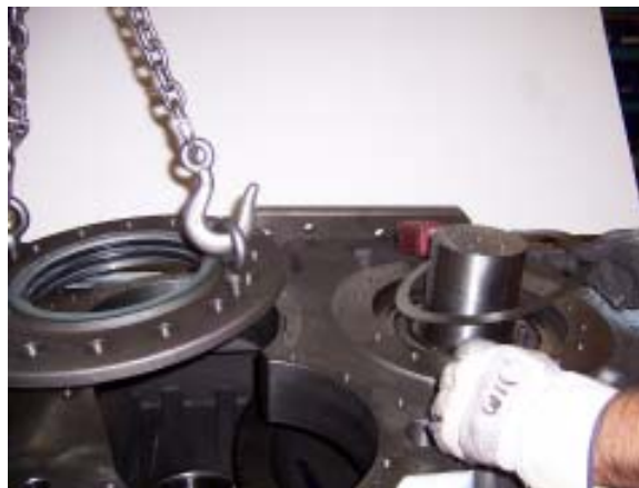
Figure 34. Removing Seal Carrier and Shims
