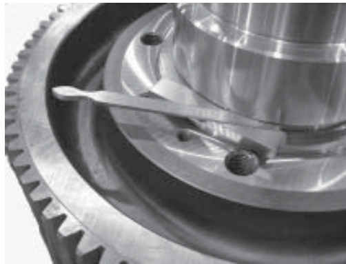
Figure 83. Measuring Output Gear Advance
