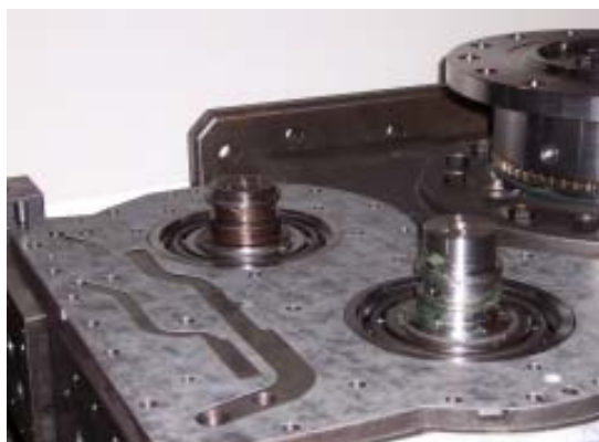
Figure 107. Bearing Cups, Spacers, and Manifold Gasket Installed
