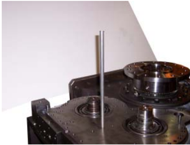
Figure 37. Lube Tube in Bearing Carrier
