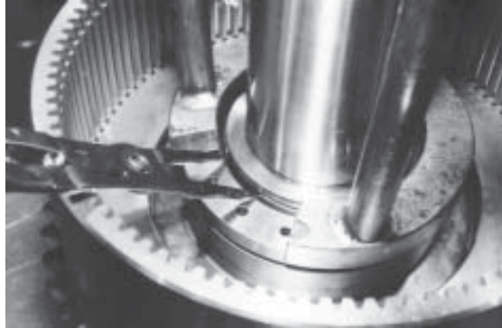
Figure 51. Removing Spring Retainer Retaining Ring
