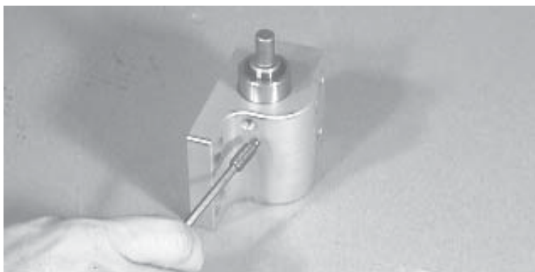
Figure 141. Installing Dogpoint Setscrew
