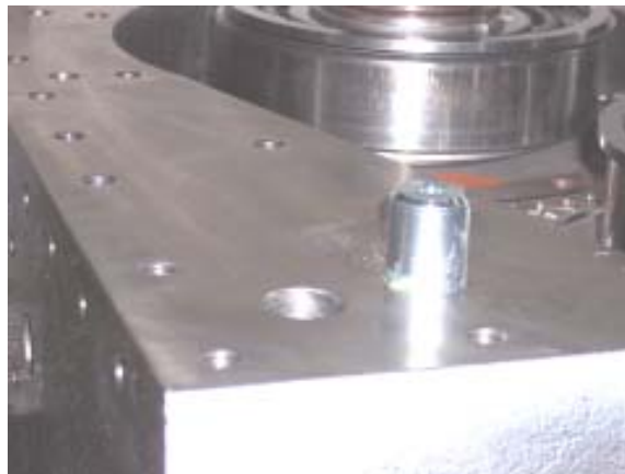
Figure 104. Lubrication Oil Pressure Relief Cartridge Installed
