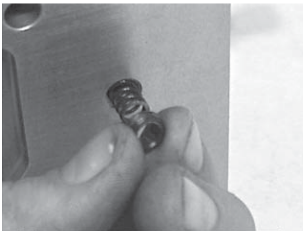
Figure 136. Installing Detent Ball Setscrew
