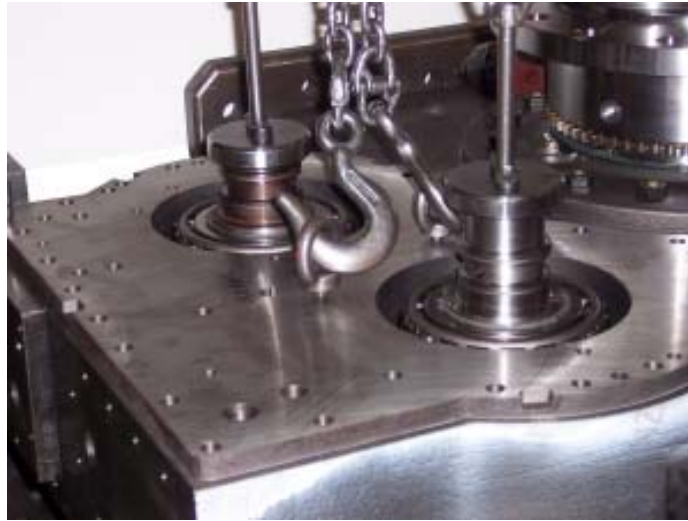
Figure 105. Install Bearing Carrier
