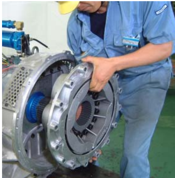
Figure 26. Removing Torsional Coupling (if equipped)
