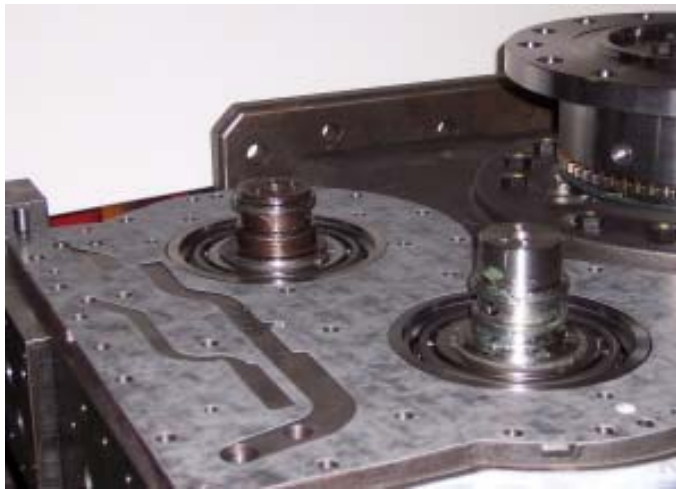
Figure 109. Install Seal Rings
