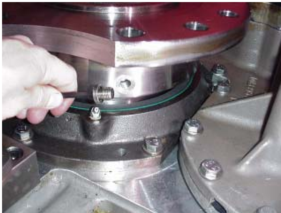
Figure 32. Output Flange Oil Injection Plug Location
