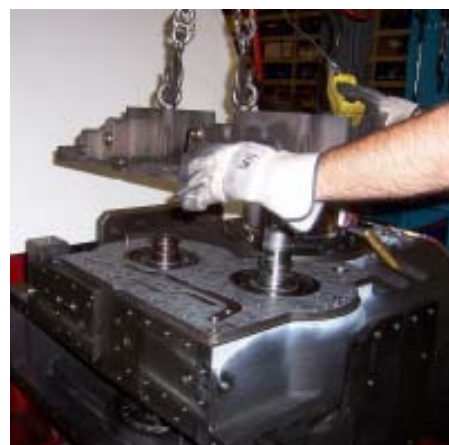
Figure 35. Pusher Screws Installed in Manifold; Removing Manifold
