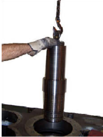
Figure 85. Installing Output Shaft
