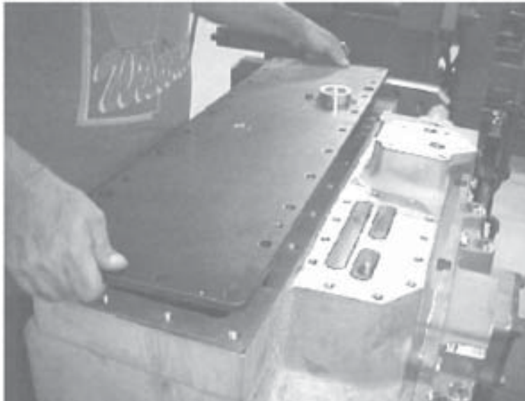
Figure 126. Installing Top Cover
