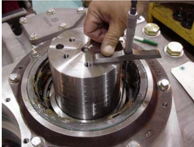
Figure 114. Measuring From Output Shaft Height
