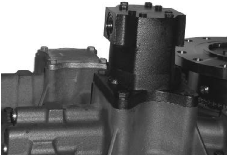
Figure 124. Oil Pump Installed
