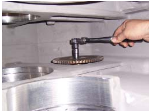
Figure 82. Securing Trailing Pump Gear to Shaft
