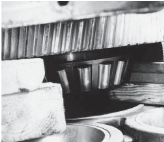
Figure 40. Supported Gear and Shaft Assembly
