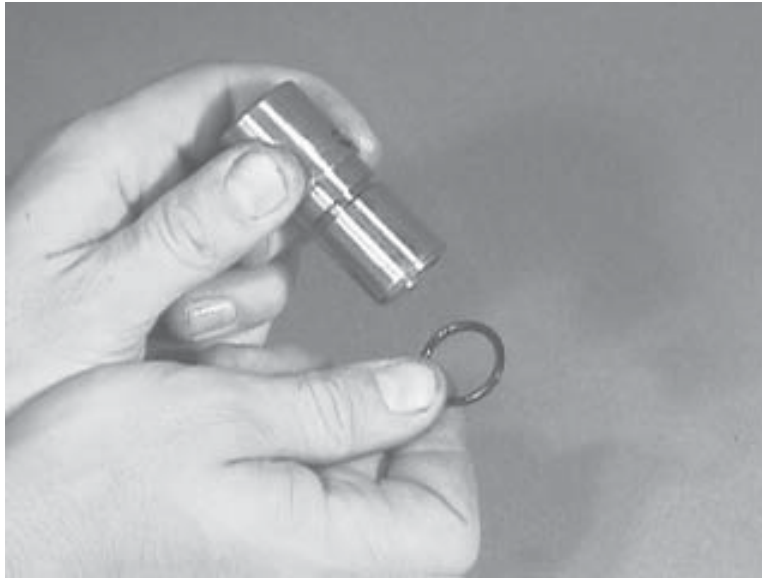
Figure 139. Installing O-ring onto Adapter
