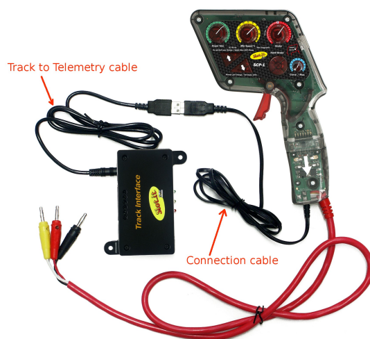
Figure 30: connection of the Track Interface to SCP controller.
