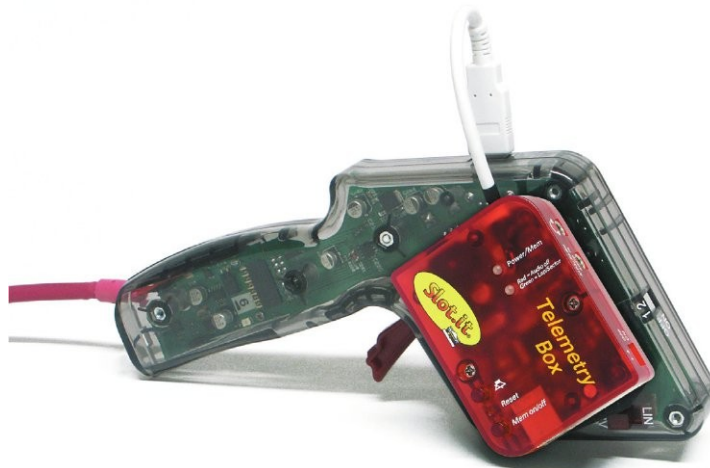
Figure 11: Universal Live Timing Box assembled on SCP controller.
