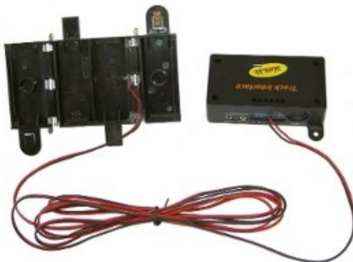
Figure 29: example of the connection of the Track Interface to a dead strip.
