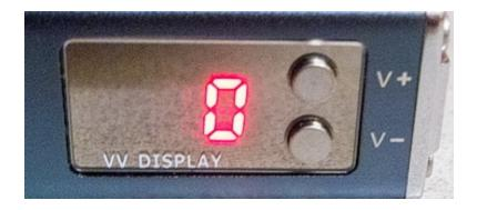
The puff counter increments upwards by one every time the power button is pressed during normal operation, regardless of how long the button is held down. The puff counter will display for approximately **1.5** seconds and then the current voltage setting will be displayed:
