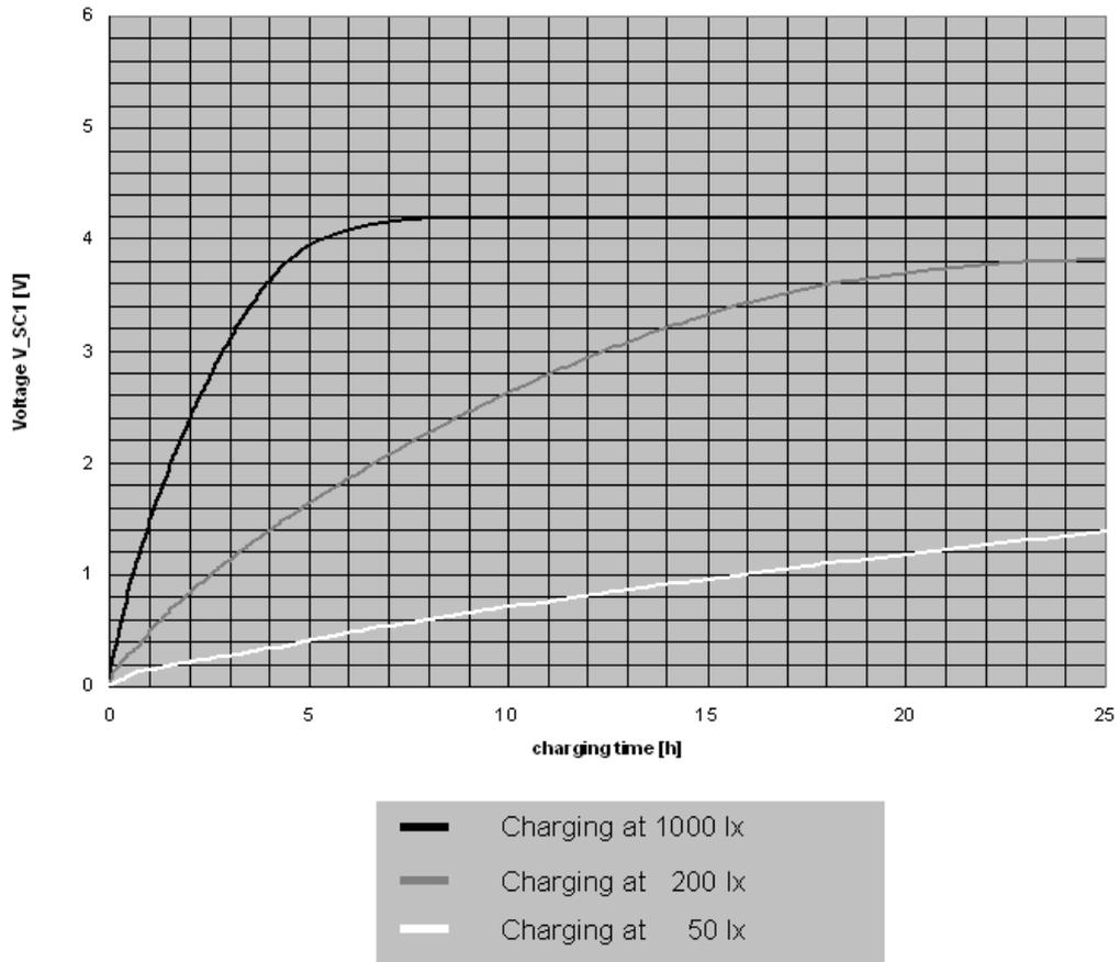
**Figure 5: Graphs of the goldcap charging process (typ. @25°C). Measured with white light LEDs, illustration of the illumination level as fluorescent lamp equivalent (EL). Measured with 100s wake up timer.**
