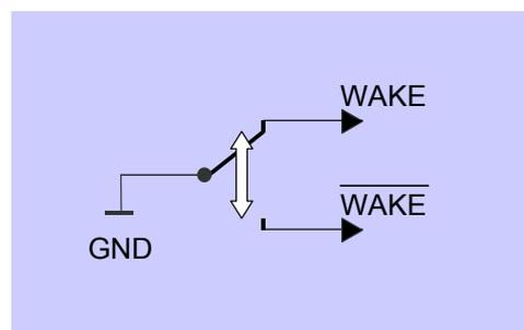
**Figure 4: External WAKE pin circuit**
