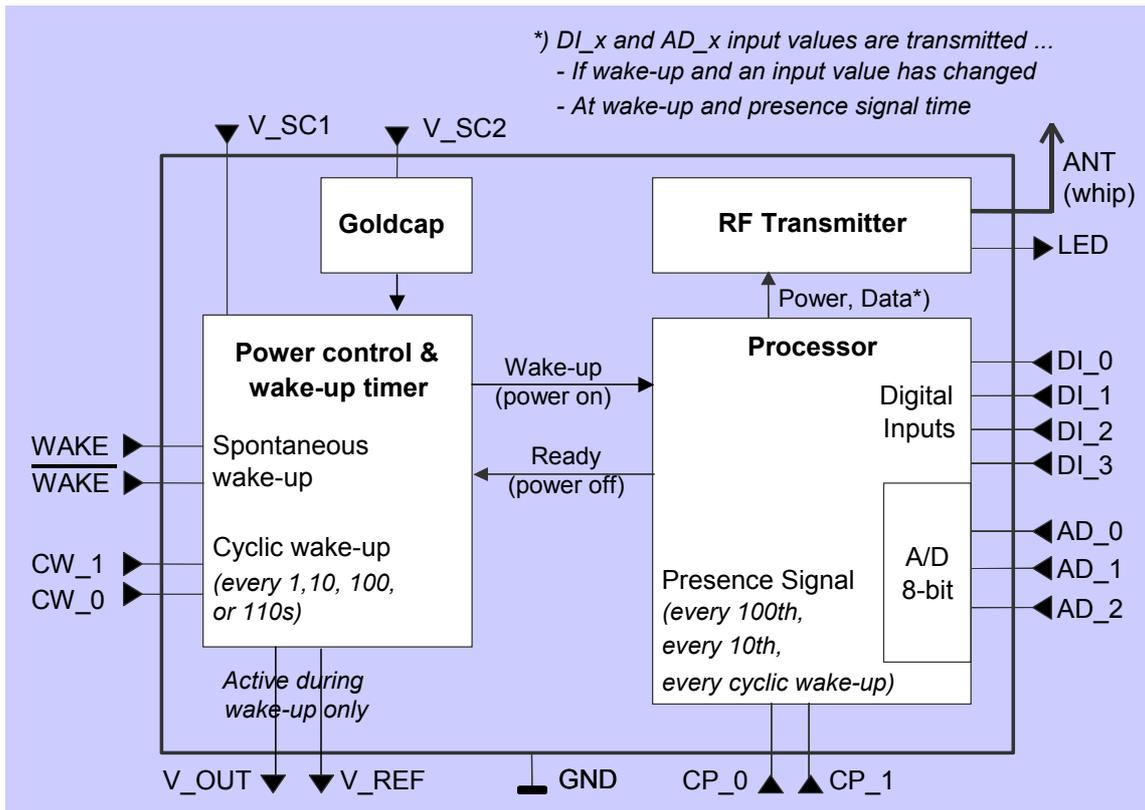
**Figure 3: STM 11x block diagram**
