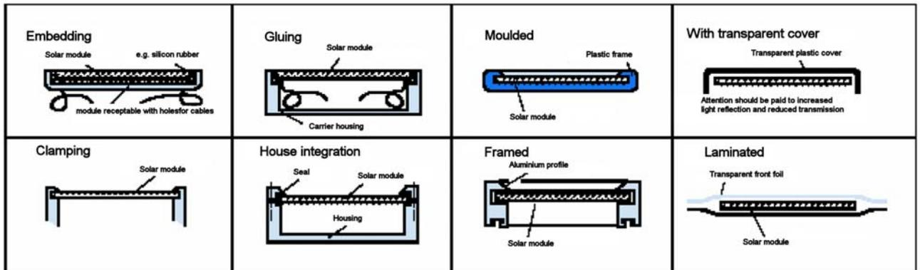
**Figure 11: Examples of solar cell mounting**
