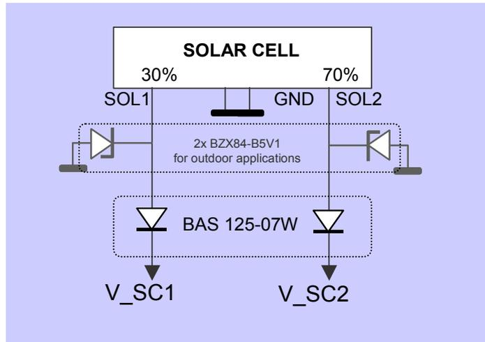
**Figure 9: Connecting the solar cell**
