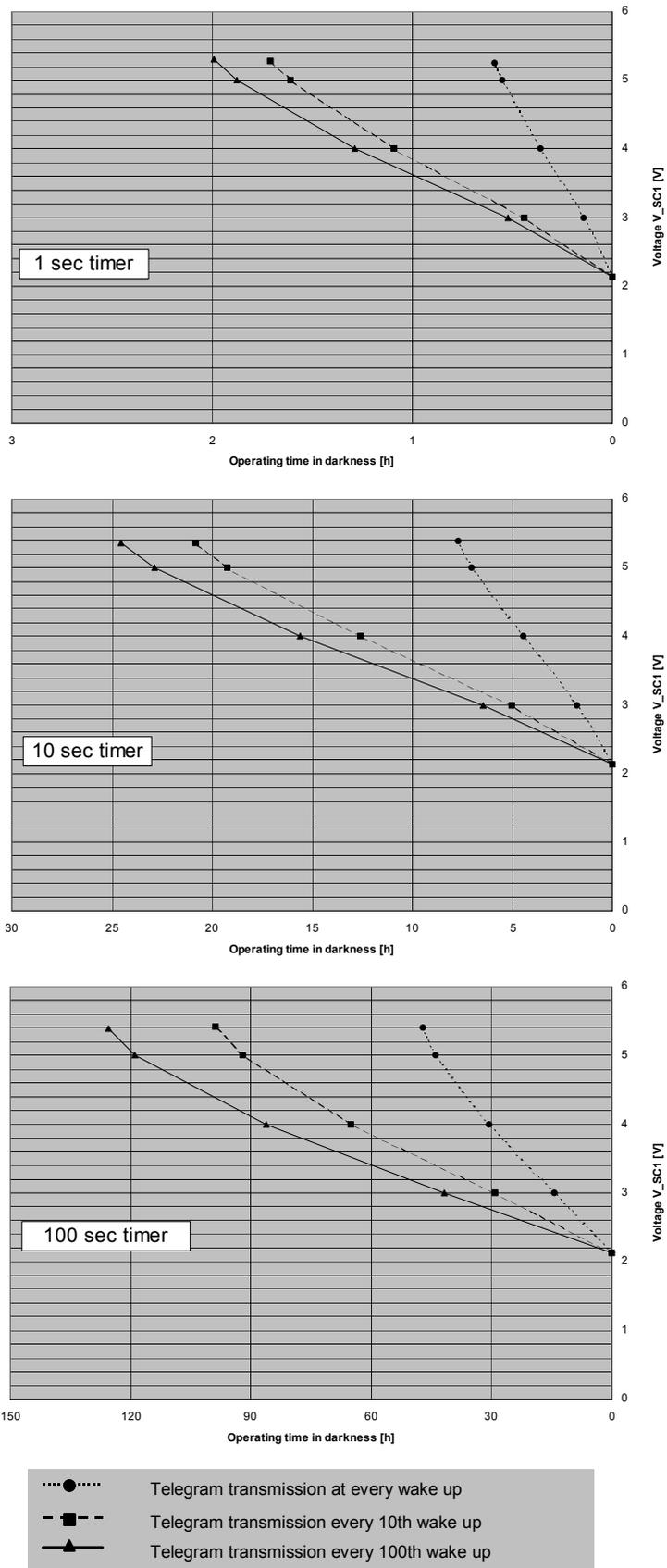
**Figure 6: STM110 operation time in darkness (typ. @25°C)**
