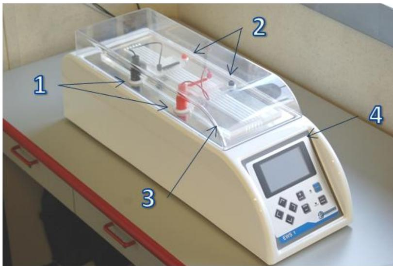
**Figure 1:** Electrophoretic WorkStation-1: 1) connectors of the high voltage module (IEF system); 2) connectors of the low voltage module; 3) safety lid; 4) control panel.
