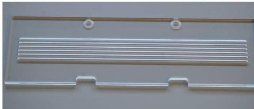
**Figure 4:** IEF tray for 42 cm long IPG strips or for shorter IPG strips of appropriate pH ranges positioned end-on-end.
