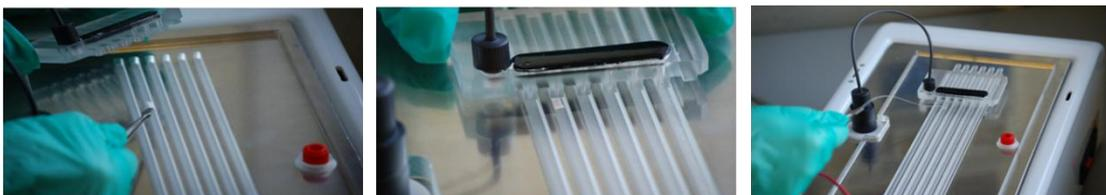
**Figure 6:** Positioning the paper bridge, the electrode and the IPG strip. These operations must be done at both the ends of the strip. Remove excess water from the paper bridges by blotting with tissue paper: paper must be only wet, not saturated or dripping.
