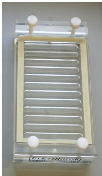
**Figure 2:** Equilibration strip tray for 7 cm long IPG strips. Other different trays are available depending on the different length of IPG strips.
