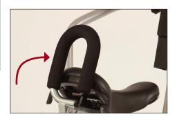
The rear stop behind the seat can be adjusted in depth. First lift up the rear stop and tilt it backwards. This reveals an Allen screw inside the U-profile When the Allen screw is loosened, the rear stop can be slid forwards or backwards in the external tube. After adjustment, re-tighten the Allen screw.
