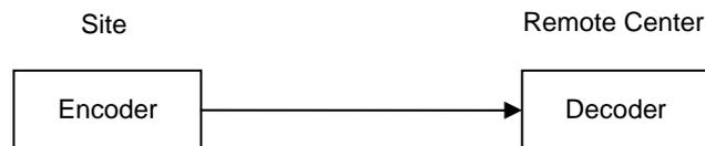
Mostly used configuration is 1 to 1 connection. An encoder is installed at a site where video images can be transmitted and a decoder is installed at a center location to receive and view the video images on analog monitor. Audio and serial data are transferred in either direction.
