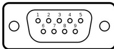
*Figure 3: CAN Bus Connector (a common DBUS-9)*
