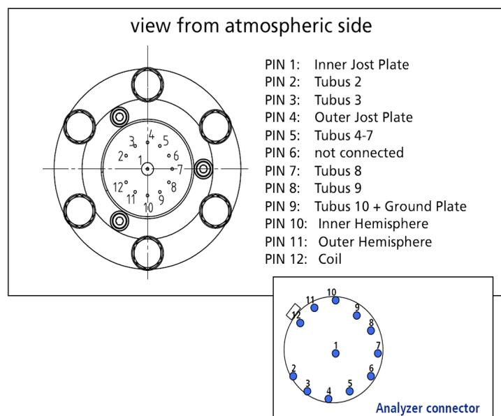
Figure 24: Schematics of the 12-pin analyzer feedthrough
