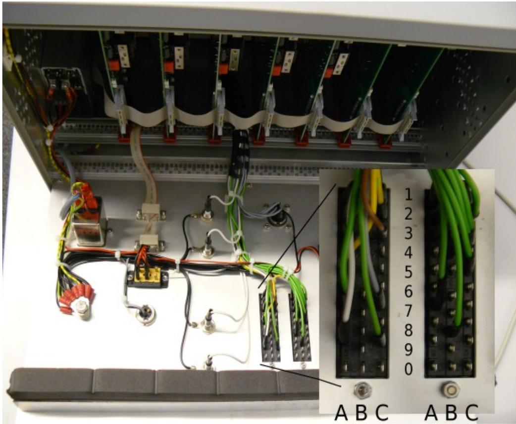
*Figure 12: HSA3500 plus with opened backplane, the pin numbers are indicated in the zoomed figure.*
