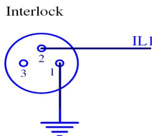
Figure 7: Vacuum interlock connector
