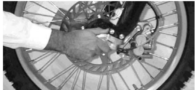
To check the steering adjustment use a stand under the chassis, and lift the motorcycle off the ground. Move the handlebar lightly to either side; if the handlebar continues moving under its own momentum, the steering is not too tight. Squatting in front of the motorcycle, grasp the lower end of the front fork (at the axle), and push and pull the fork (as shown on the previous photo); if free play is felt, the steering is too loose.
