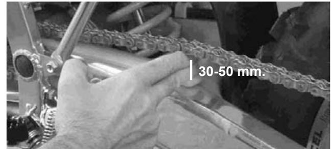
In addition to checking the slack, rotate the rear wheel to inspect for damaged rollers, loose pin and links, unevenly or excessively worn teeth, and damaged teeth.
