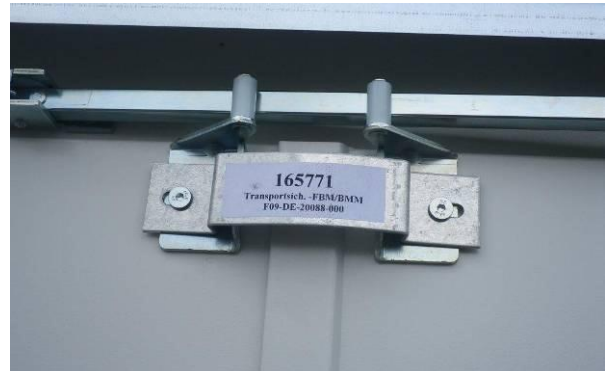
Fig. 3-2: with transport securing device
