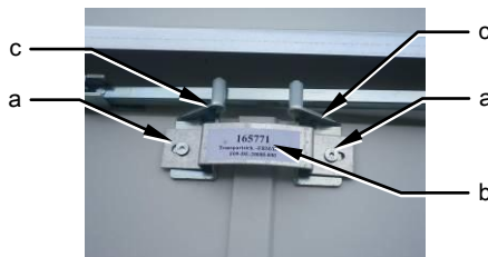
Fig. -34: Winged door – transport securing device
