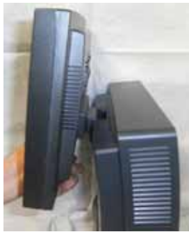
a. Mount the Second Display module onto the base cover
