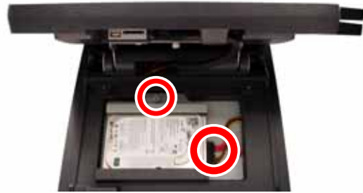
b. Loosen the thumb screw of the HDD bracket (1) and release the SATA cable to replace HDD kit.
