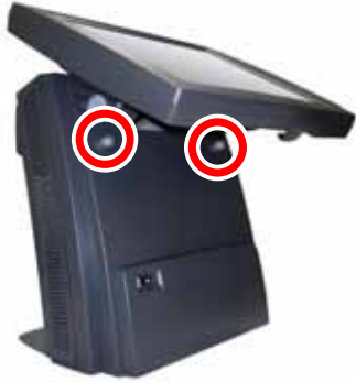
a. Loosen the thumb screws (2) and release the front cover.
