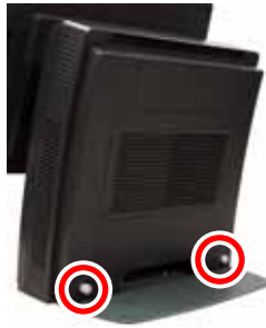
a. Loosen the thumb screw (2) to release the base cover
