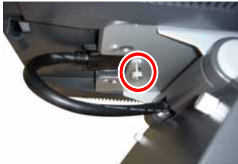
a. Loosen the metal bracket thumbscrew (1)
