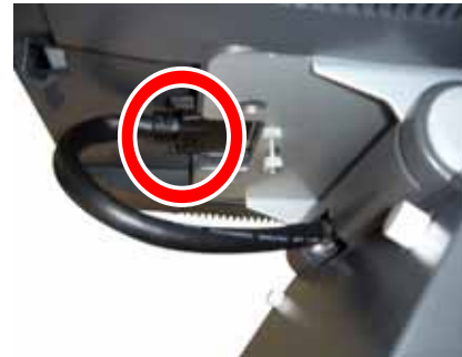
b. Loosen the I/O cable screws (2)
