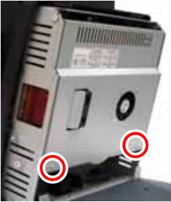
b. Loosen the screws (2) to release the metal shielding cover.
