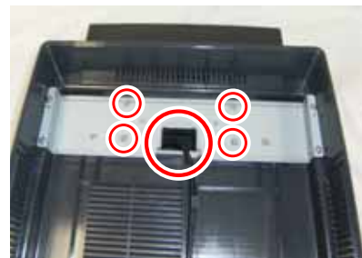
b. Tighten the screws (4), connect the VGA cable to the second display and route the VGA cable as shown in the picture.
