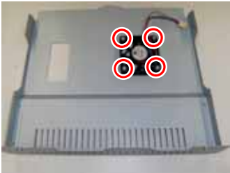
d. Loosen the screw (4) to replace the system fan
