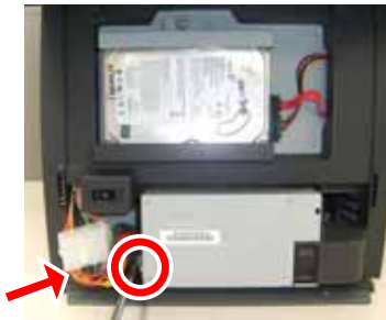
a. Loosen the screw (1) and disconnect the power connector
