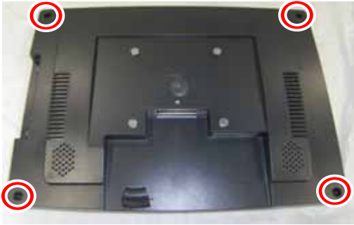
a. Loosen the screws (4) to release the LCD cover
