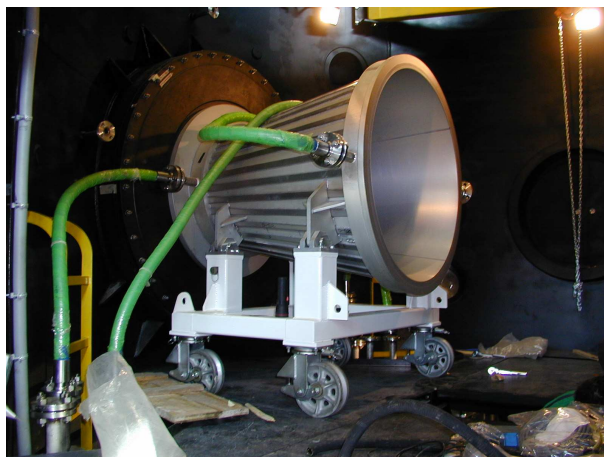
Fig. 12: Conical nozzle mounted into Test Chamber (1150 mm exit diameter configuration).
