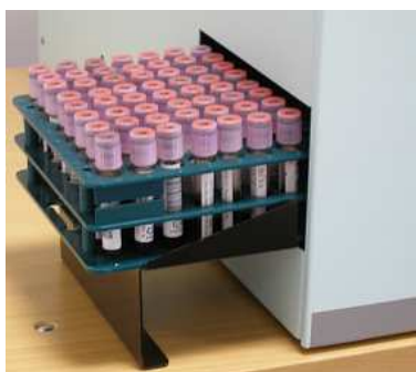
Fig. 2.2.2 left side of the Ves-Matic Cube 200 (exiting sample holder rack)
