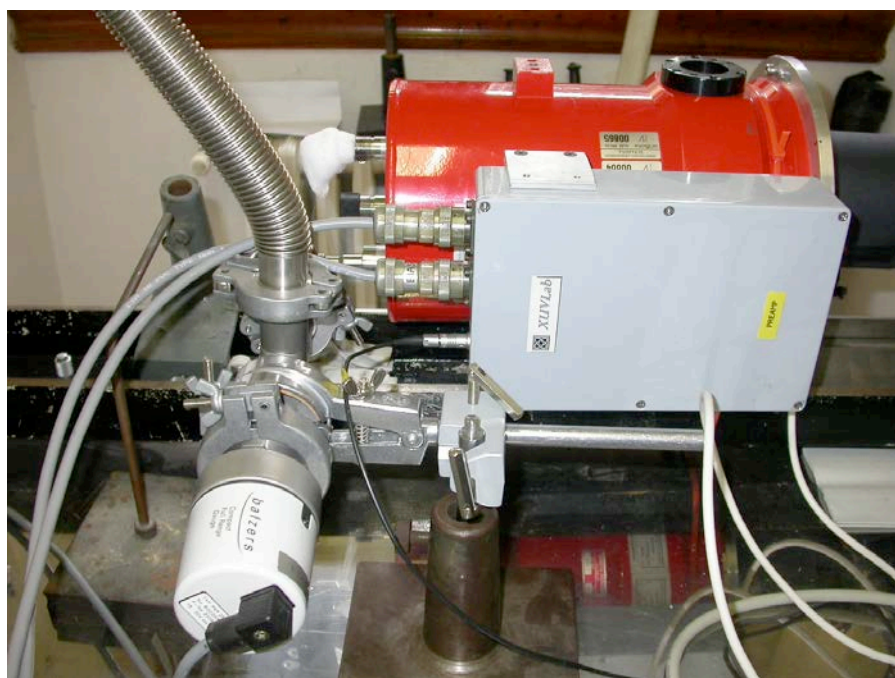
Figure 2.1.b. The LN2 dewar with the proximity electronics hosted in the grey box.
