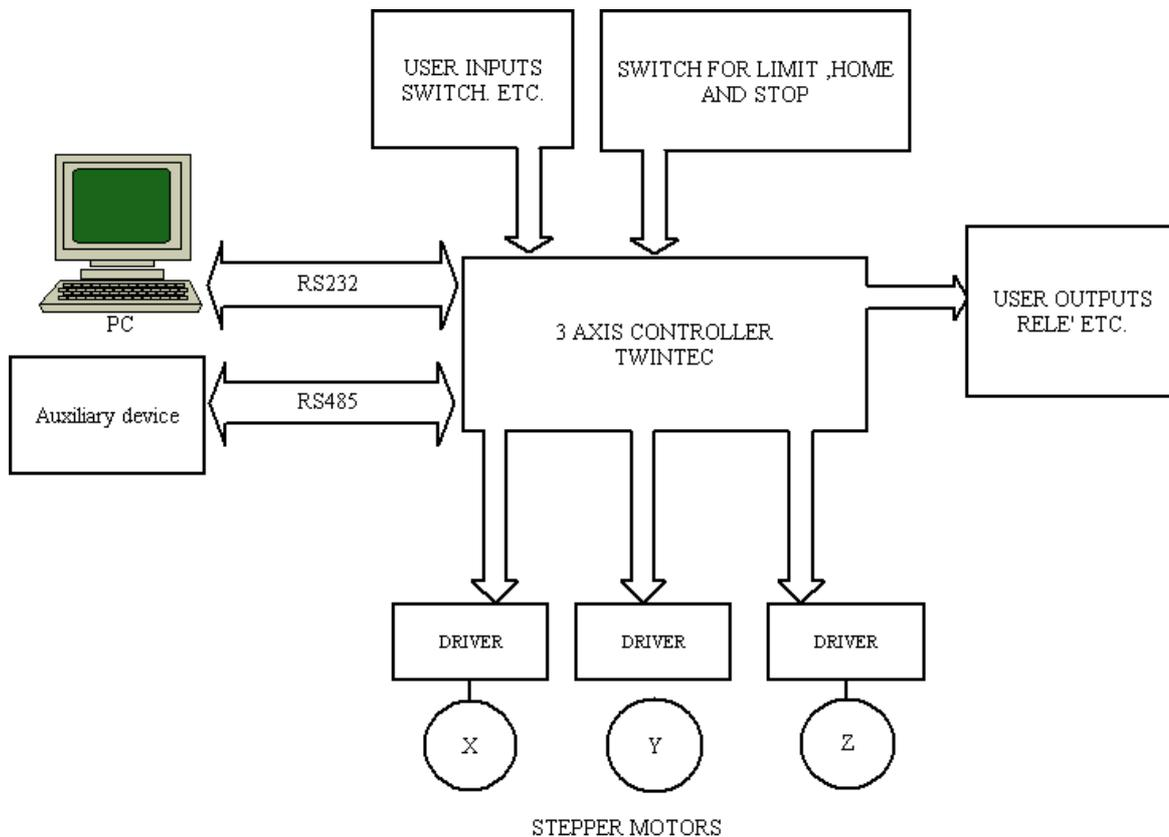
The controller is the head of a positioning system. It perform the following tasks:
