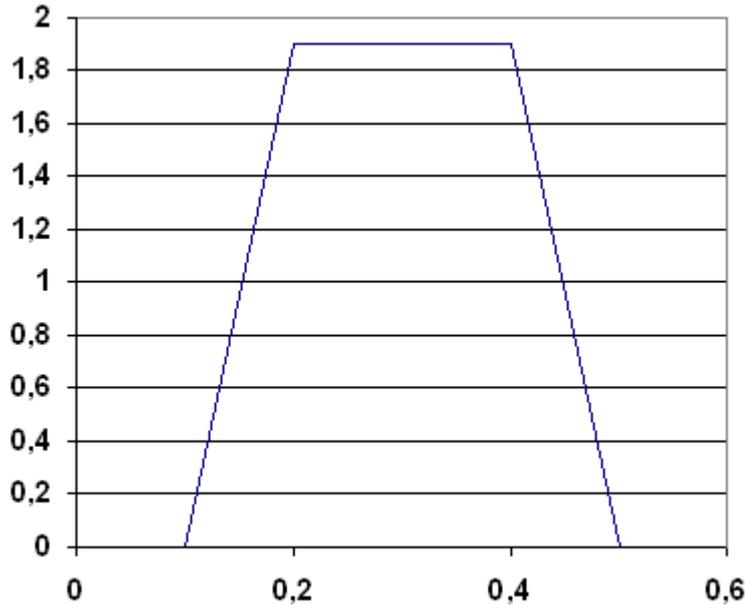
If the length of the vector is too small to reach the final velocity the form of the curve is a triangle.
