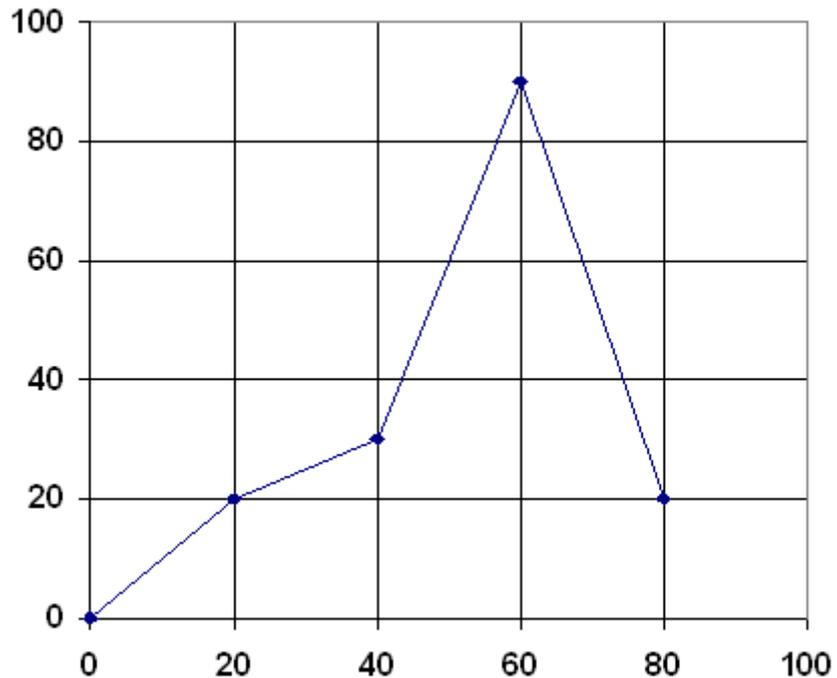
If the contouring angle is set to  $23^\circ$  (default value) the execution of that path is done with 3 accelerations and 3 decelerations. This because the angle between the first and the second vector is less than  $23^\circ$  while the angle between the second and the third vector and between the third and the fourth is greater than  $23^\circ$ .
