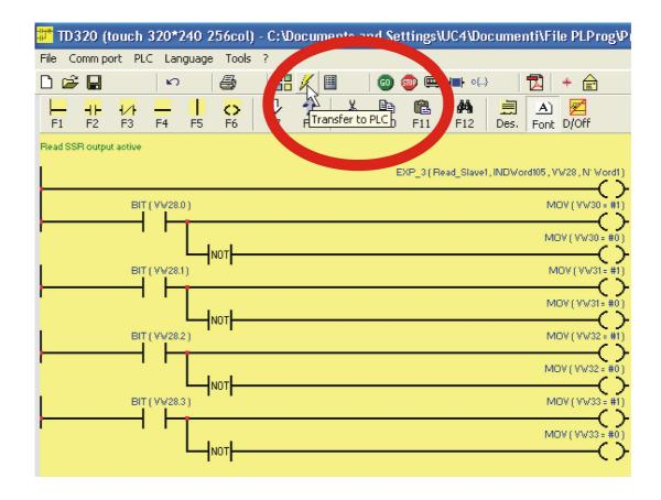
If the TD320 is connected correctly to the PC (see diagram of **section 4.1**), during the transfer the terminal will show this figure on the display:
