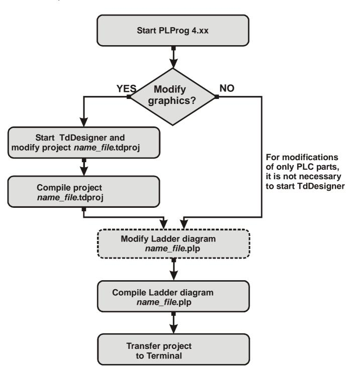
For eventual modifications of only the PLC part (as outlined) it is not necessary to start TdDesigner. The compilation of the project file\_name.plp will maintain the graphics unchanged and will activate the modifications of the Ladder diagram.
