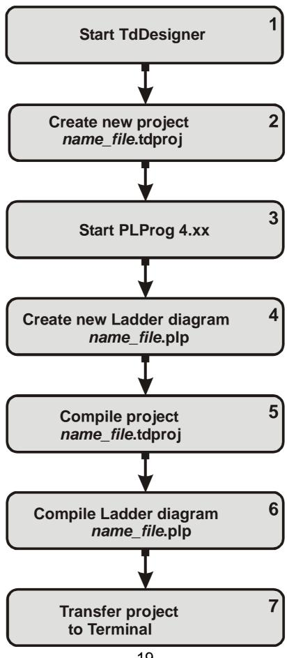
To create a new project and transfer it to the terminal, follow the procedure and described below:
