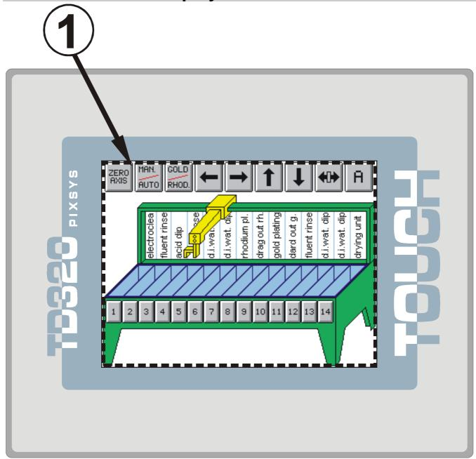
1 DISPLAY Type: Back-lit LCD, resistive touch screen STN Dimensions: Active Area 5.7"
