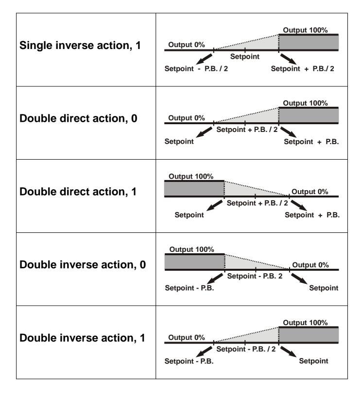
The PID function, for correct operation, must be called at the most regular intervals possible, thus by timer, or for more brief and precise times, by an internal interrupt.
