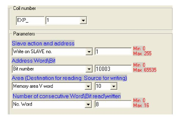
The following illustration, however, reads the register DATA REGISTER of the PLC NAIS, the 10 words from DT0 to DT9, and copies them in the area of V0 to V9 of the TD320.
