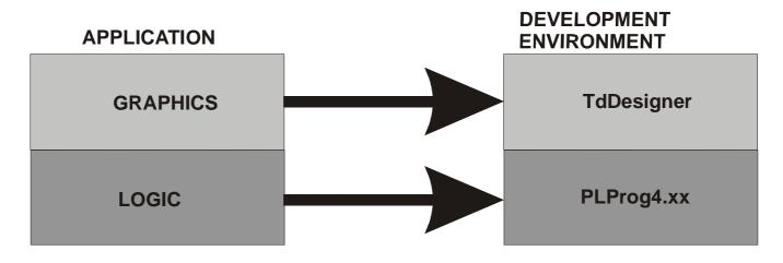
Any application managed by the TD320 terminal should therefore be realized using both the development environments, **implementing therefore two different files** strictly connected between them.
