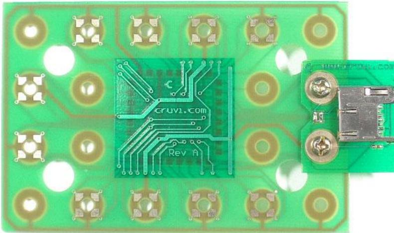
Baseboard ready for boot from micro-SD Card (power adapter board not shown).
