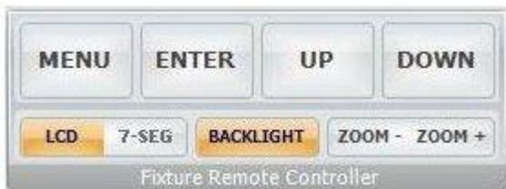
This panel emulate the display panel of each fixture present in the network. Fixtures not equipped with any display will be emulated through a 7 segment display.
