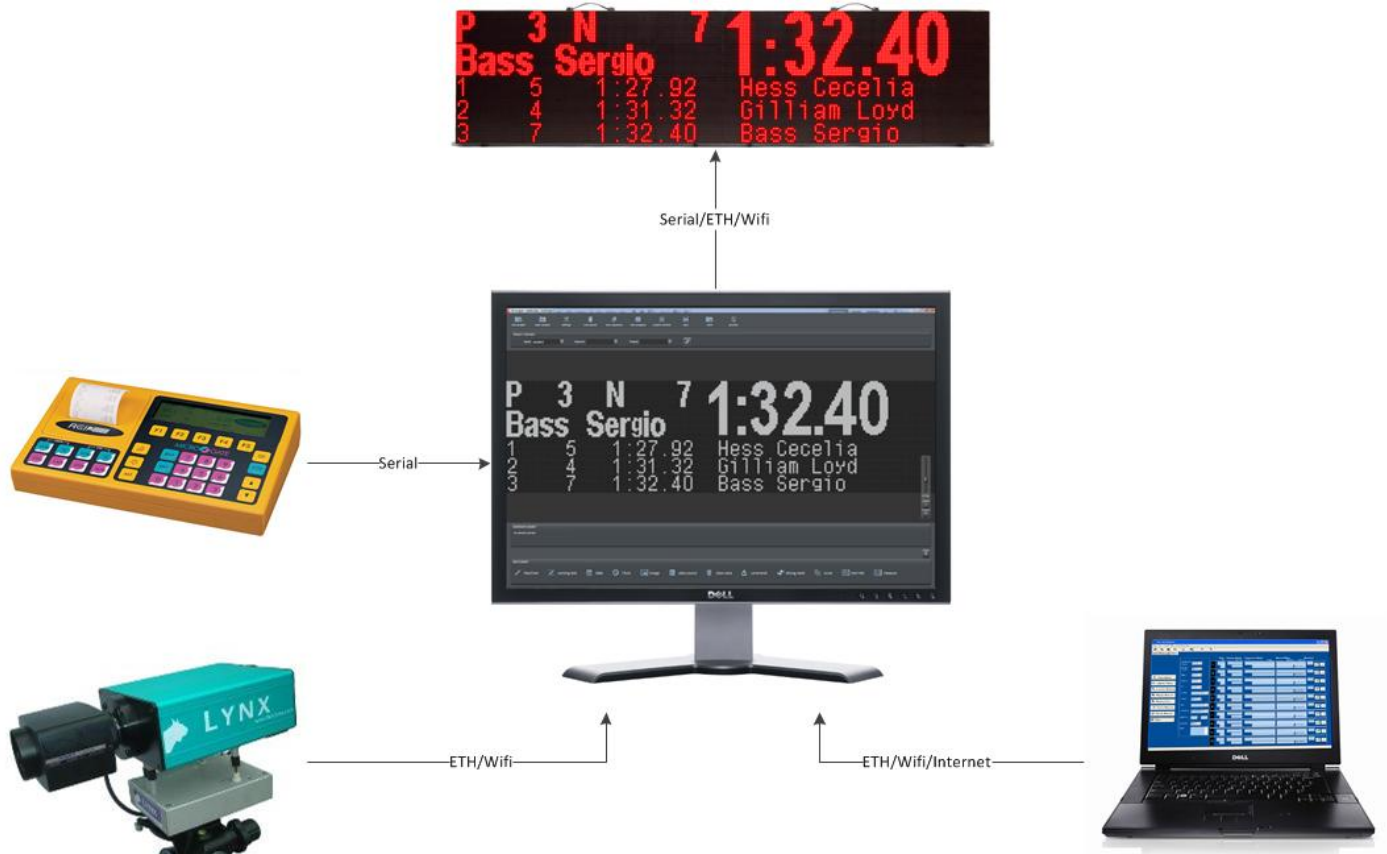
Figure 2 - various Data Sources connected with .netBoards
