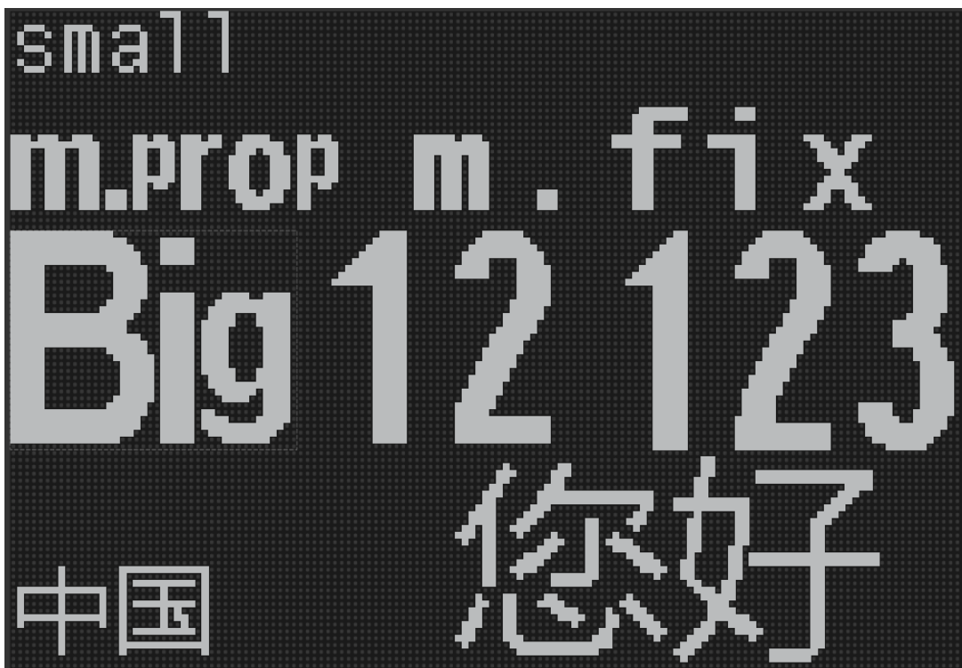
Figure 17 - Font examples: small, medium prop, medium fix, large, special1, special2, unicode medium and unicode large
